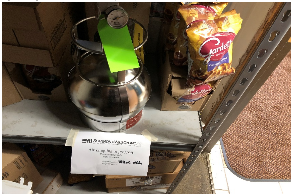
Exhibit 3-2: Indoor air sampling in progress inside the store closet (IA-02 sample location)
