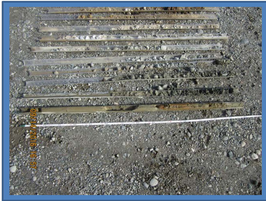
Photo 3: View of lithology in Boring B-1-2016. Top left at ground surface. Bottom right at 50-ft bgs. Each liner is 5 ft in length. (September 14, 2016)
