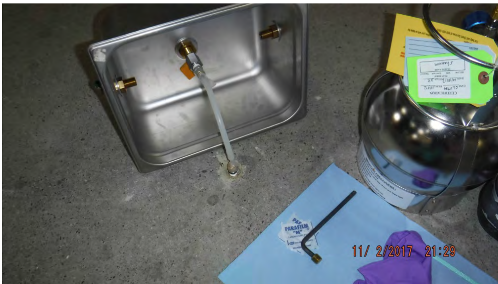
Photo 14: Assembling the soil-gas sampling apparatus inside the service station garage. (November 2, 2017)
