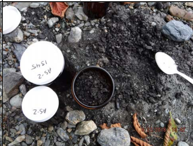
Photo 4 – Collecting asphalt sample for SPLP-VOC/SVOC analysis. Date: 8/23/18. Time: 1342.
