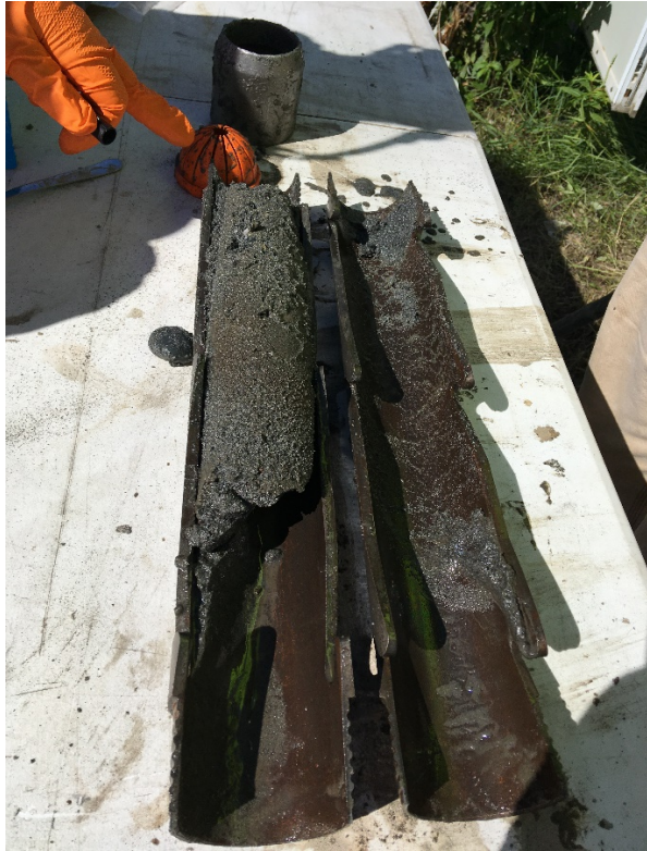
Soil Sample collected in Split Spoon Sampler
