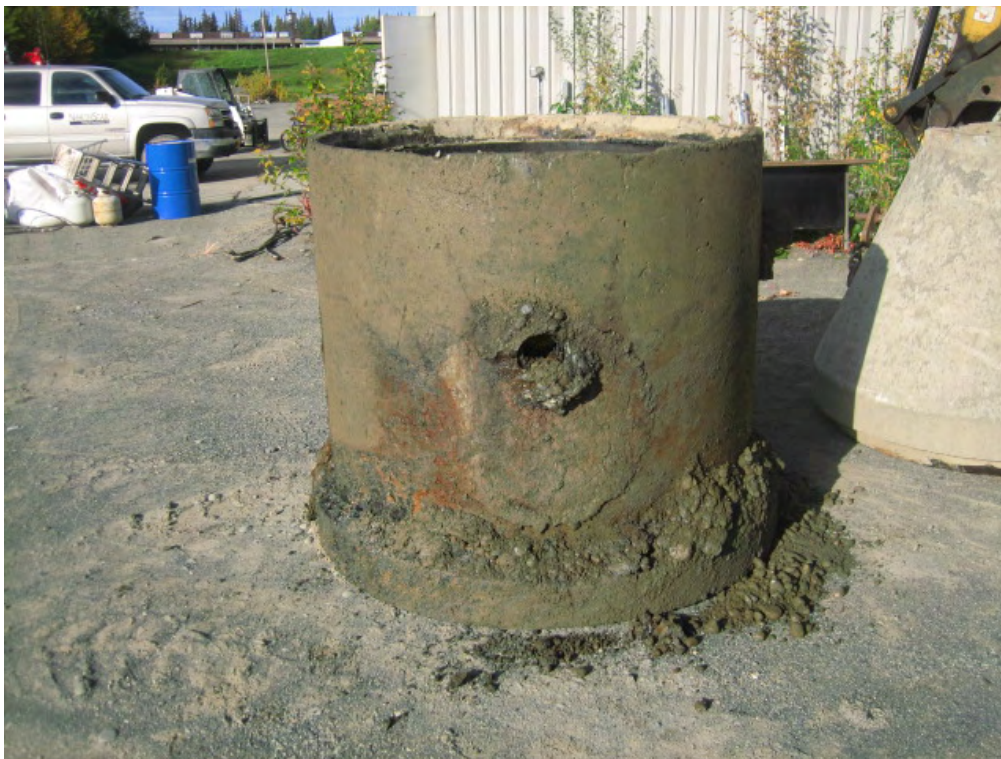
Photo 6: Base section of oil/water separator tank removed. Red and black staining on exterior below outlet invert for approximately \frac{1}{4} of tank circumference.
