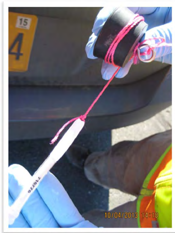
Photograph 3 – Close-up of module# 716776 tied to the black rubber stopper with string.
