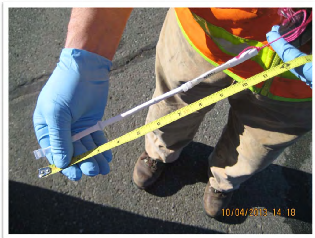
Photograph 4 – AGI Universal Samplers were 11 inches long when uncoiled.
