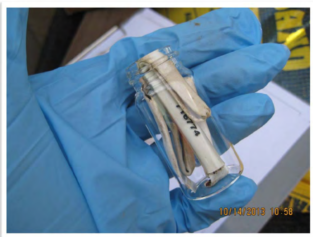
Photograph 8 – Upon retrieval after 10 days of deployment, Universal Samplers were returned to the lab in glass vials.
