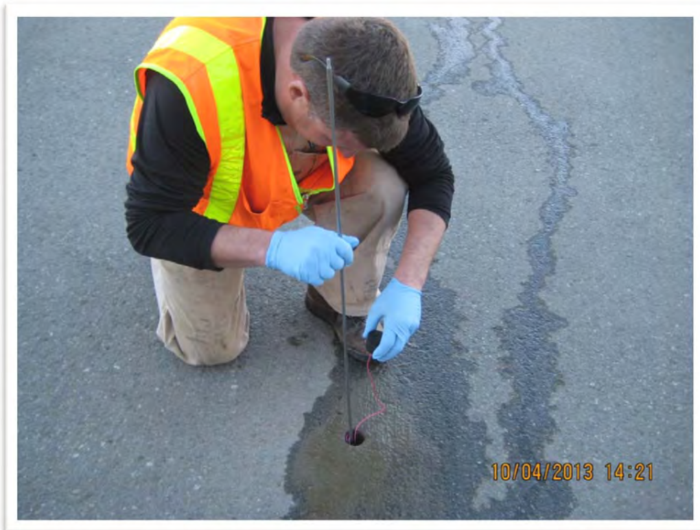
Photograph 6 – An insertion rod was used ensure the Universal Samplers were at the bottom of each hole.
