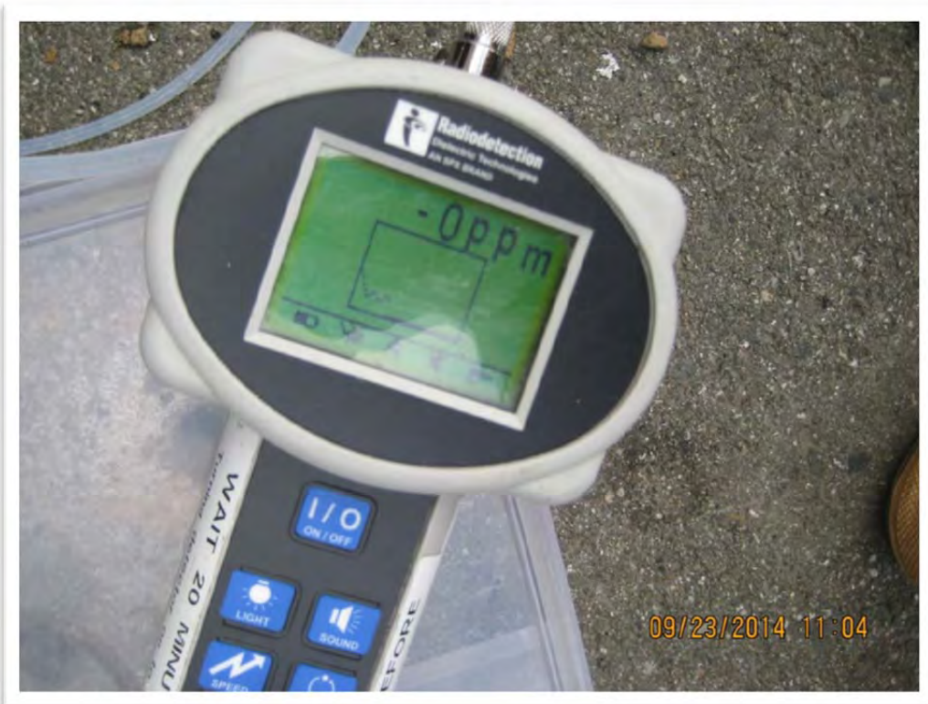
Photograph 8 – Instrument used to measure the concentration of helium in parts per million.
