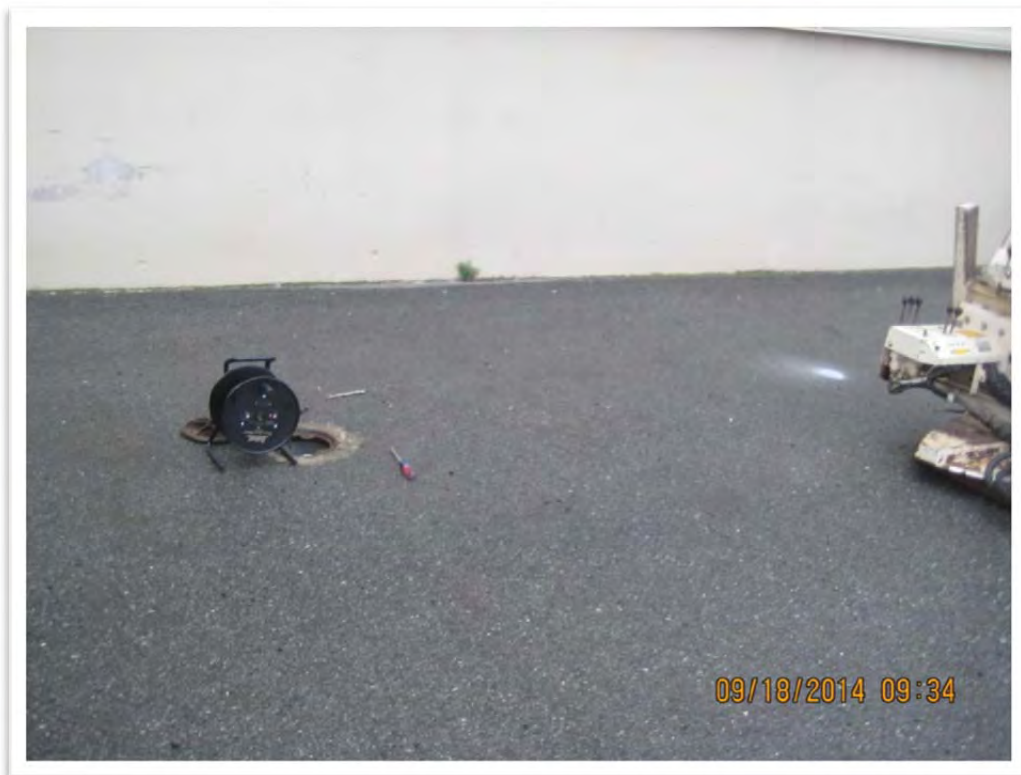
Photograph 2 – Water levels were measured in adjacent existing wells to determine depth of soil gas monitoring wells; boreholes were advanced to approximately 1 foot above the water table. View to the north.
