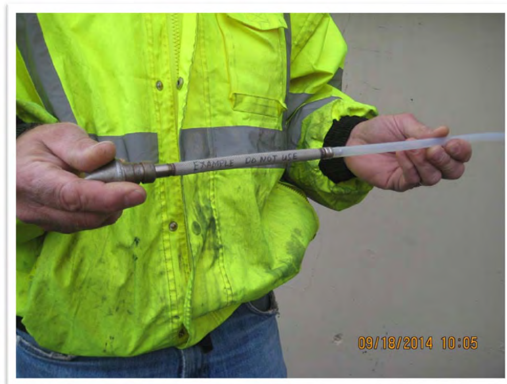
Photograph 4 – Example of Geoprobe 6-inch-long stainless steel implant connected to Teflon-lined tubing used in the construction of the soil gas monitoring wells.
