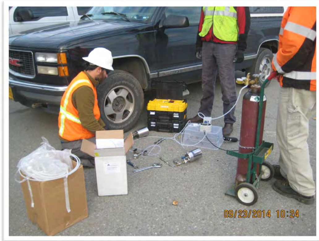
Photograph 7 – Leak tests were performed prior to sample collection using helium as shown here. Samples were collected in 1-liter stainless steel Summa canisters (both primary and field duplicate are shown).
