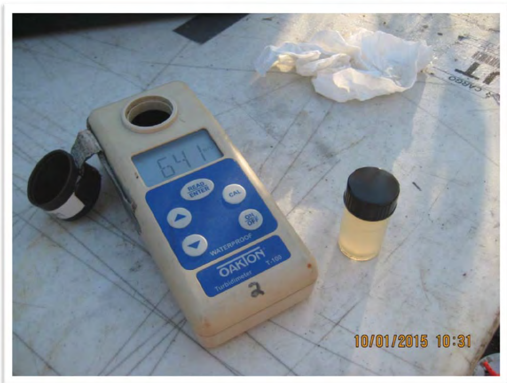
Photograph 6 – Turbidity reading logged during development of well MW-7.
