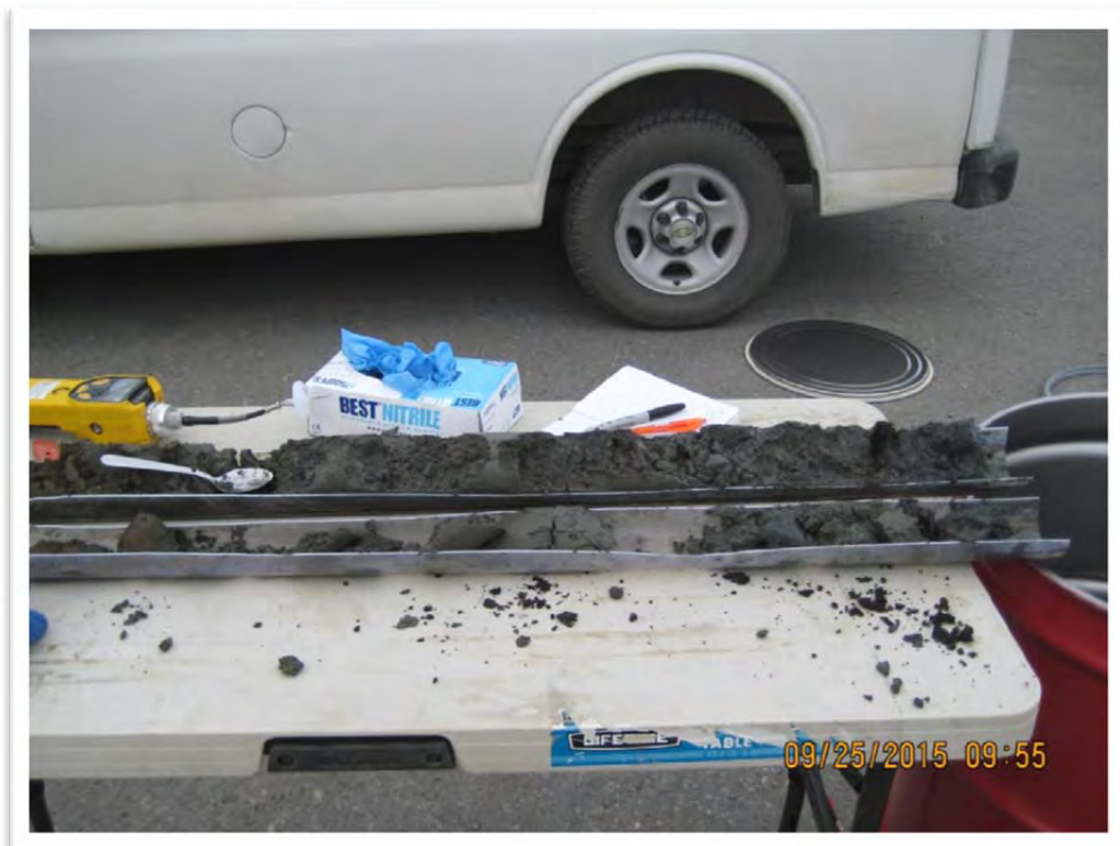
Photograph 2 – Soil cores were logged, screened, and sampled. Cuttings were placed in drum to right of photograph.
