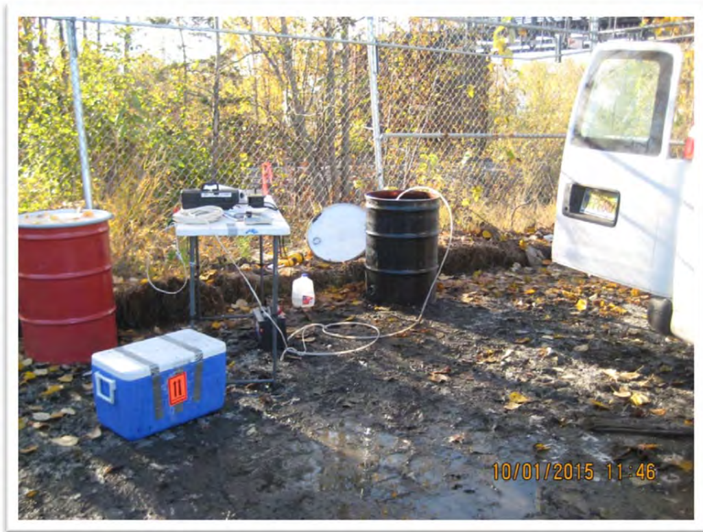
Photograph 5 – View of well MW-6 during well development. Purge water was containerized in 55-gallon drums and disposed of through the National Response Corporation. View to south.
