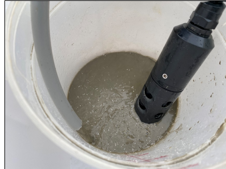
Groundwater from monitoring well RSE-15
