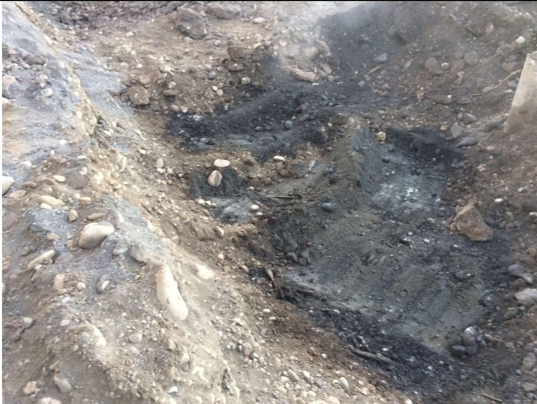
Photo 2: Sandy layer found under the burned debris. Looking Northeast (10/21/2017)
