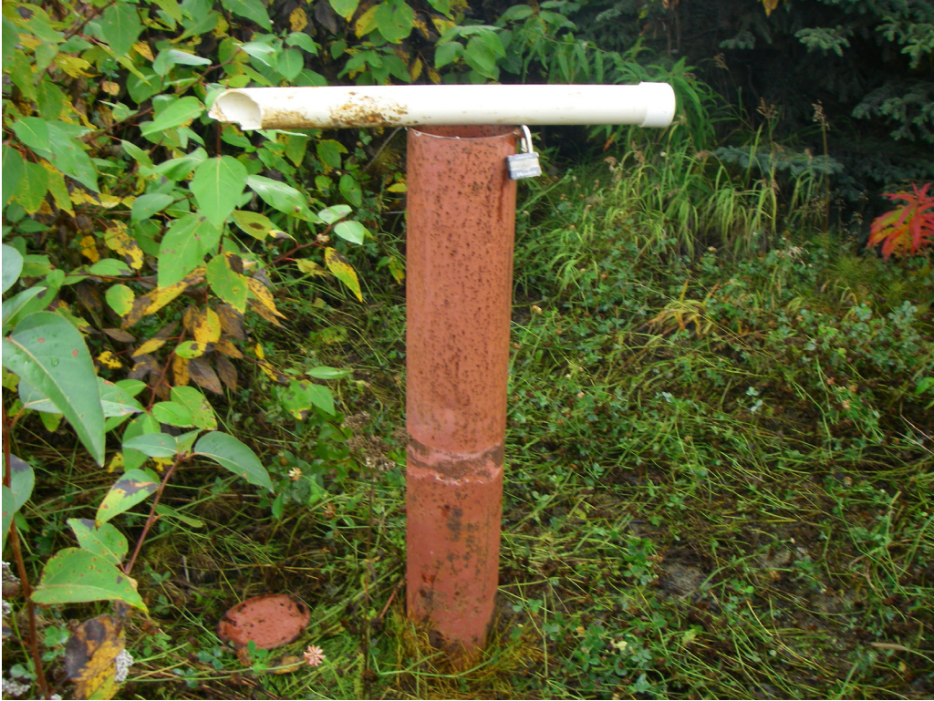
Photograph 1: GW-1 with broken casing piece.
