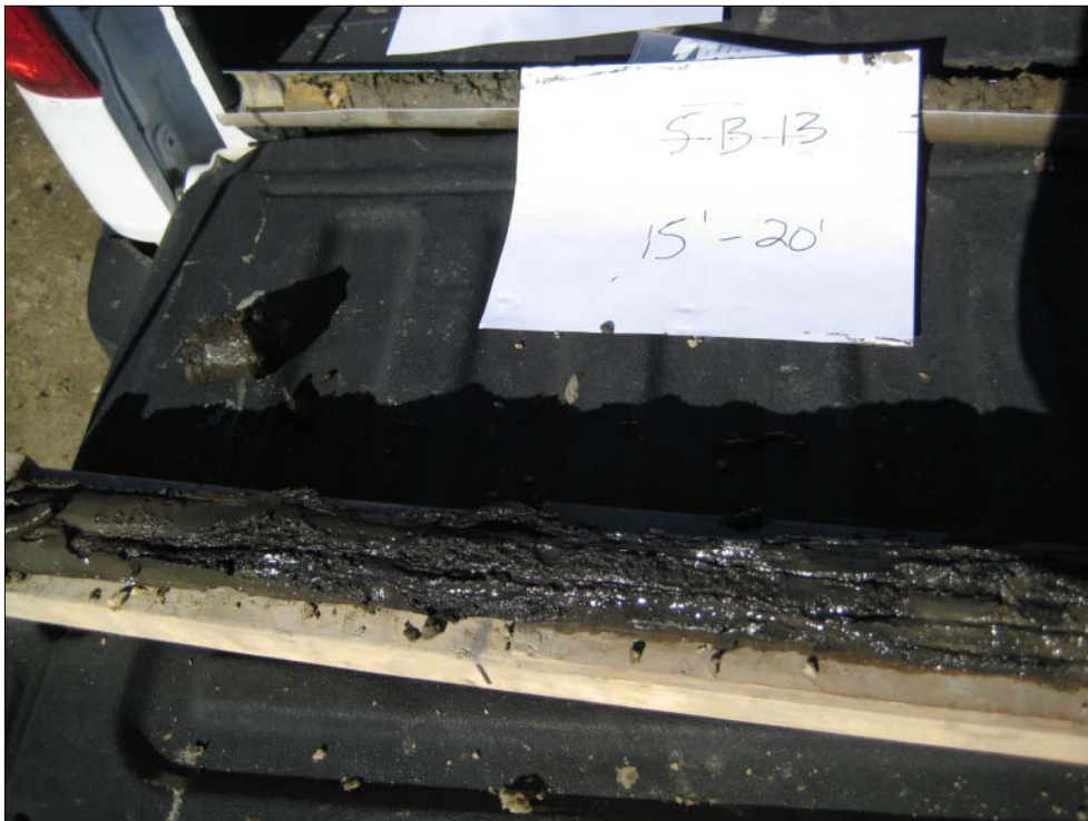
Photo 04 - Recovered soil core from 15-20 foot depth of SB-13, moist/saturated fine silt with organics, but is too fine to produce water
