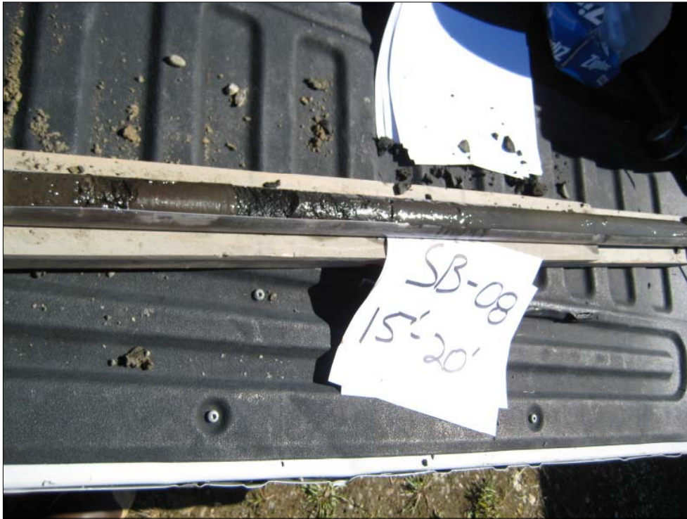
Photo 05 - Recovered soil core from 15-20 foot depth of SB-08, frozen fine silt with organics
