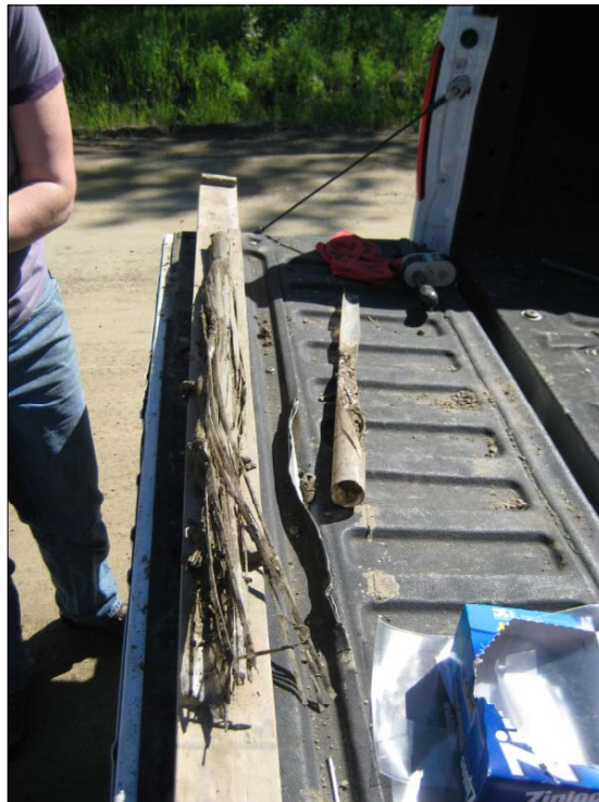
Photo 06 - Shattered soil core sleeve with no recovery in frozen silt
