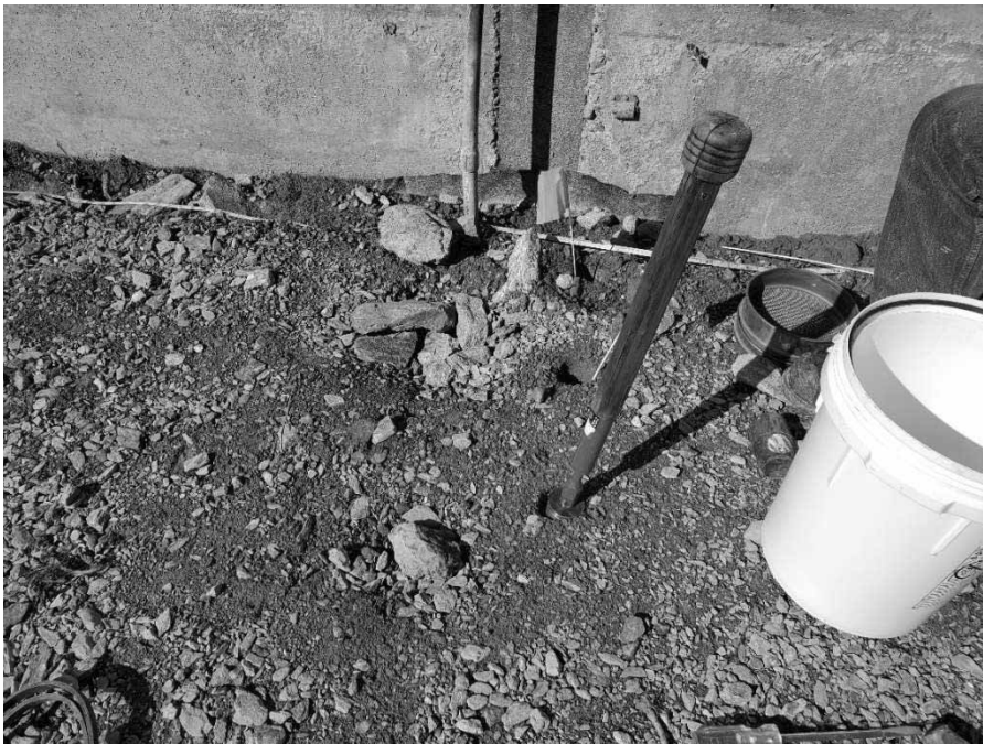
Photo 6: Collecting 12-inch core samples at 1 ft., 2 ft., and 3 ft. off the wall.
