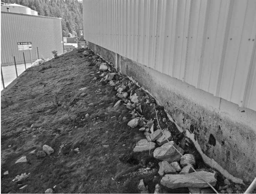
Photo 3: Flags marking approximate sample locations in DU2 (CSB Southeast). Note fill material is primarily rocks, significantly hindering sampling.
