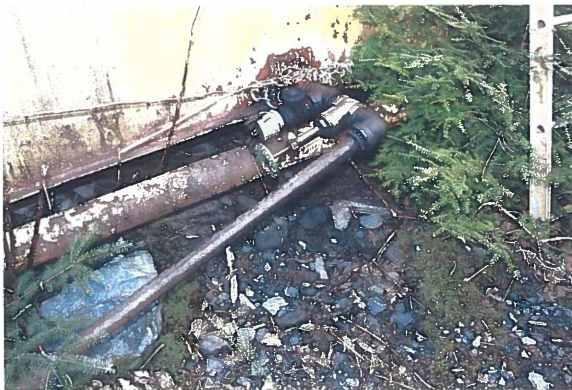
Photo #8: 3/26/12 view of the Wrangell Lumber fuel depot's 20,000-gallon diesel oil tank outlet, showing oil-stained soil where NORTECH sample #TF3 had a high DRO level of 8,110 mg/kg.
