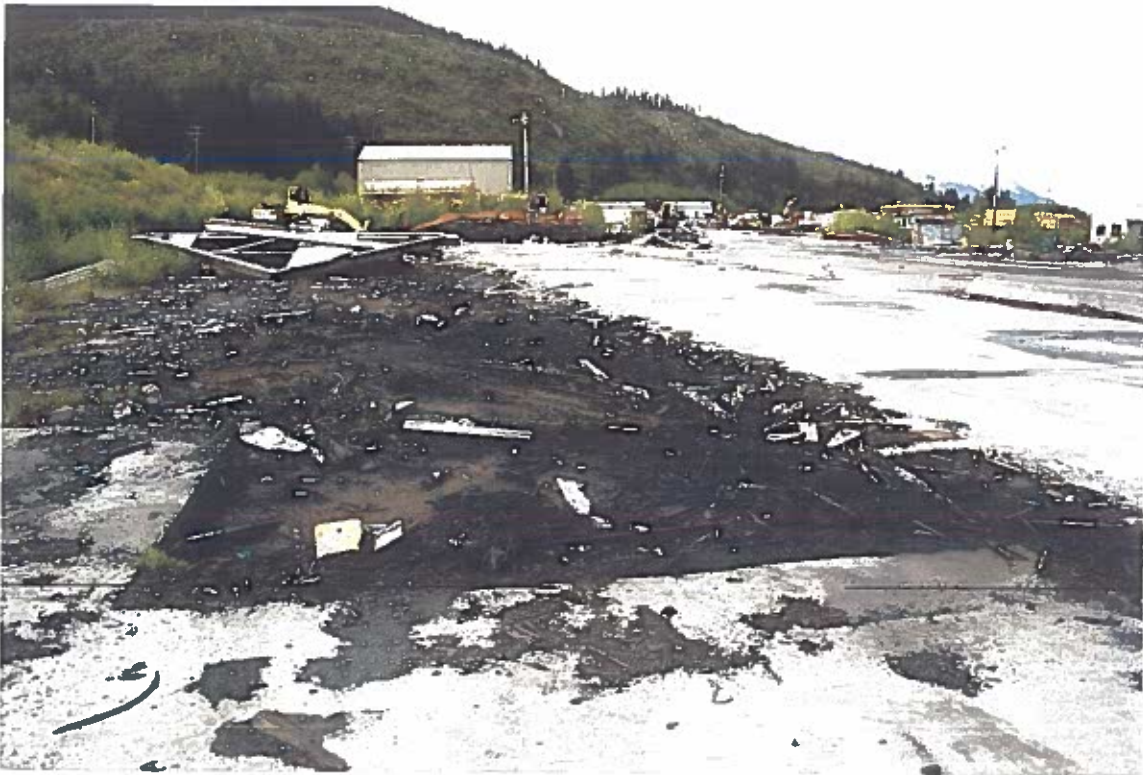
Photo #27: 5/19/12 view looking south across the Wrangell Lumber mill's former green chain area, where dark-stained soils were found extending along the edge of the concrete foundation. Oil-contaminated soil was found in several shallow hand excavations.
