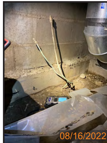
PHOTOGRAPH 6: VIEWED EAST- ABANDONED FUEL LINES IN CRAWL SPACE & PID SREENING BELOW VAPOR BARRIER
