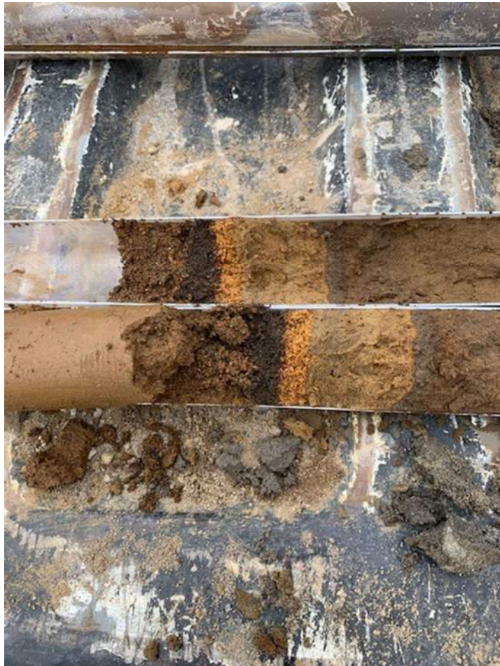
Photo 4: Possible volcanic layers observed from 6.5 to 7 feet bgs in SB-10.
