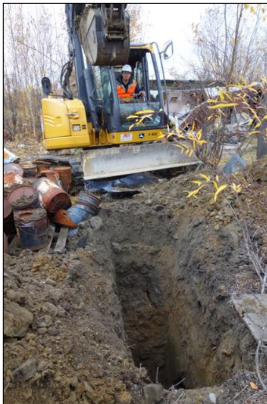
PHOTOGRAPH 36: DIG PIT (TP-25) IN STAINED AREA OF INTEREST #1; PID READING OF 10 PPM; COLLECT SOIL SAMPLES (SS-7A AND 7C) AT 1FT AND 6.5FT BGS FOR VOCS AND METALS ANALYSES; LOOKING EAST. 9/22/16.
