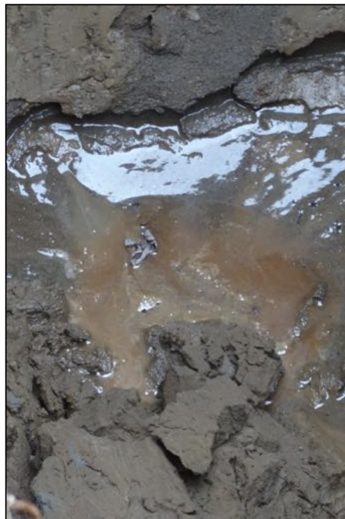
PHOTOGRAPH 38: TEST PIT (TP-25) IN AREA OF INTEREST #1 IS EXCAVATED TO GROUNDWATER DEPTH OF 6.5FT BGS; POSSIBLE SHEENING OBSERVED ON WATER SURFACE. 9/22/16.
