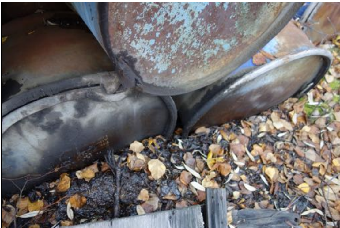
PHOTOGRAPH 26: LEAKING DRUMS CONTAINING LITHIUM GREASE LOCATED IN WESTERN PORTION OF SITE PID READING OF 10 PPM; (SEE FIGURE – AREA OF INTEREST #10). 9/22/16.
