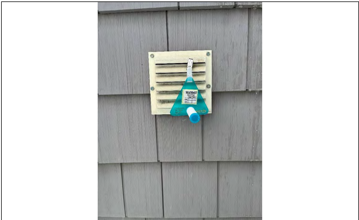
Photo 2: Outdoor air sample taken in vicinity of Fresh 80 vent on unit 138A. Date: 2/3/2023
