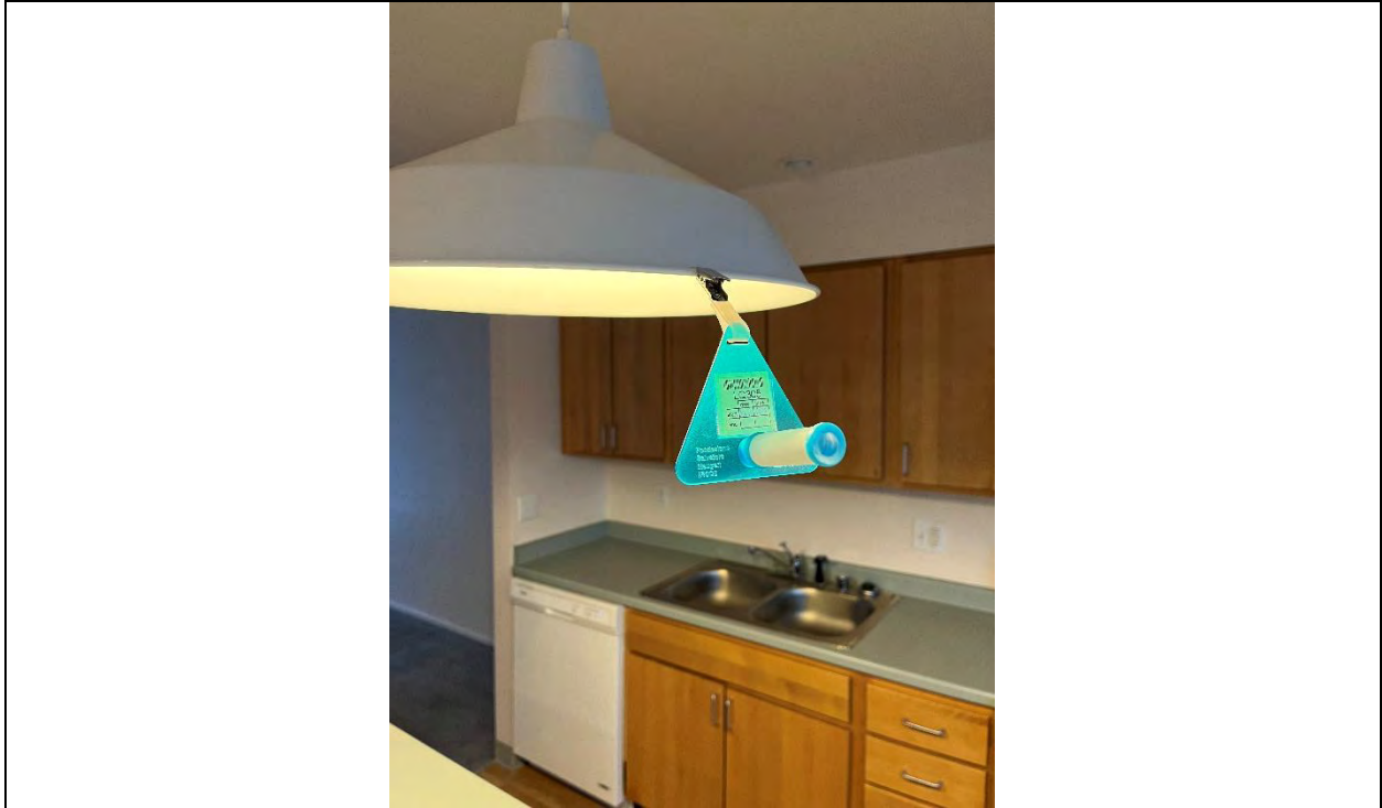
Photo 1: Indoor air sample on the second story (main floor) of unit 146B Date: 1/13/2023
