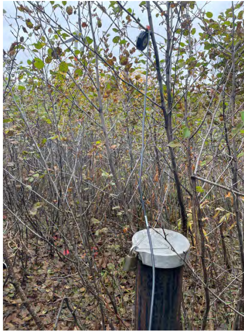
Photo ID: BE004. View north. MW-19RRS-R secured with lock, tall alders encroaching. GPS antenna hanging above well in the alder.
