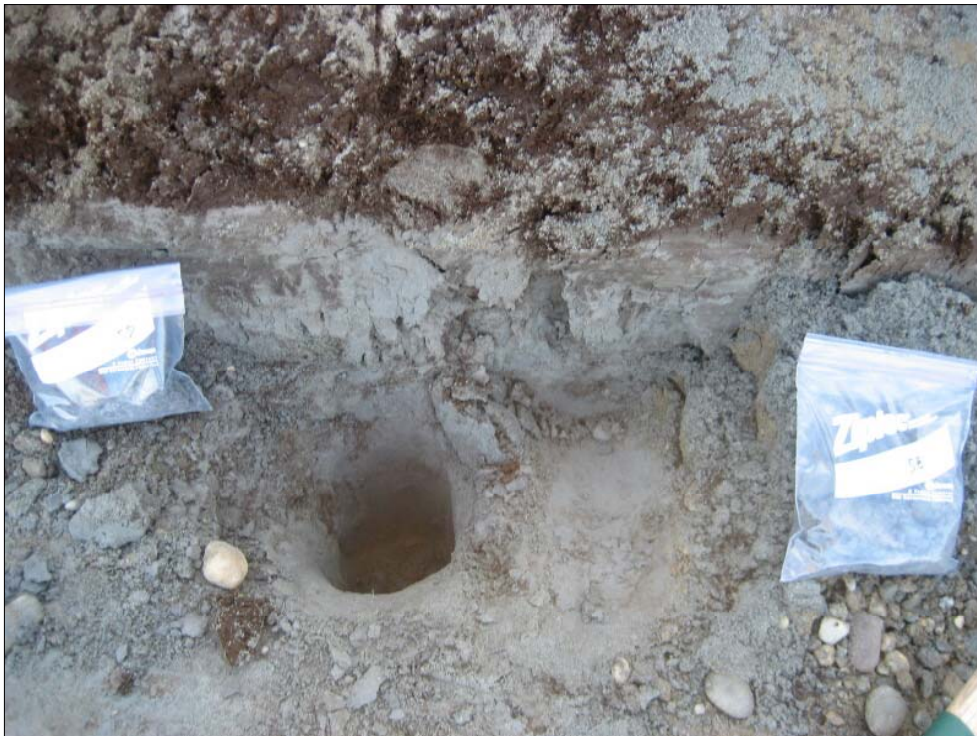
Photo 8 - Field screening of bottom southern excavation limits
