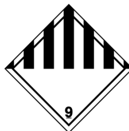
Example placard (Miscellaneous Dangerous Goods)
