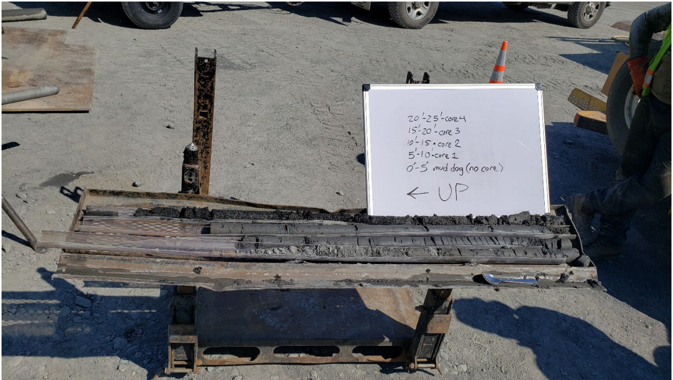
Photo 2: Direct push soil cores from SB1. A dry sandy gravel overlies over 10 ft of silt with intermixed gravel interpreted to be dredged backfill from the harbor. Wet gravelly sand was present at the bottom of the borehole interpreted to be native beach material (5/27/2022).
