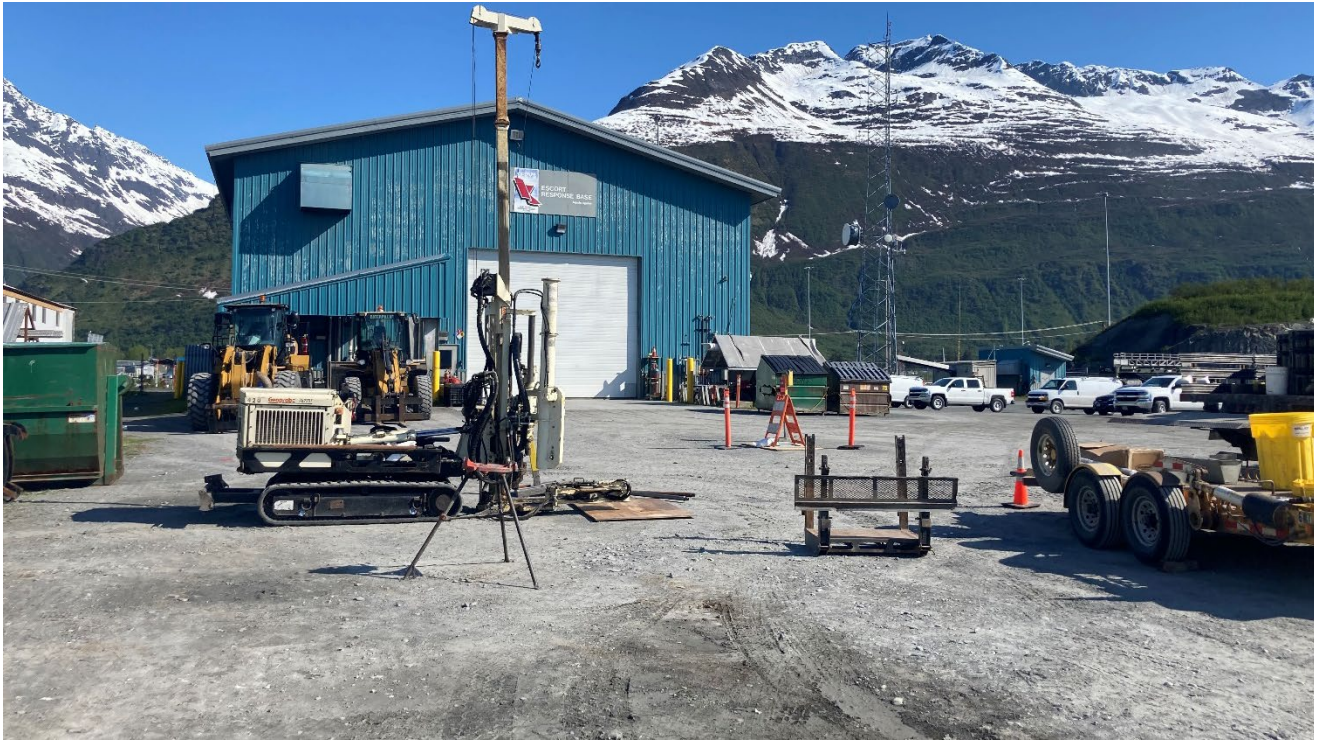
Photo 1: Advancing borehole SB1 south of the Valdez Emergency Operations Center (VEOC) Building using direct push tooling. View to the north (5/27/2022).
