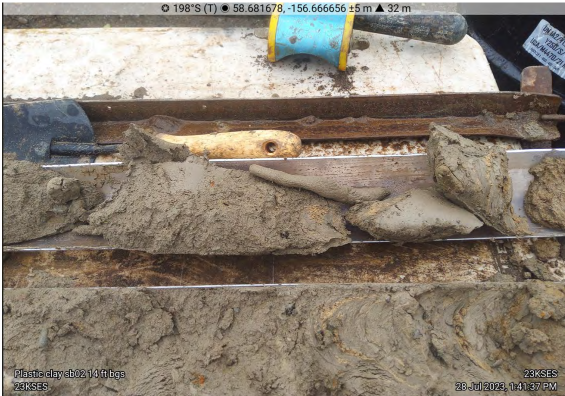
Photo 11. SB-02 14 ft bgs, plastic clay. Date: 7/28/2023.
