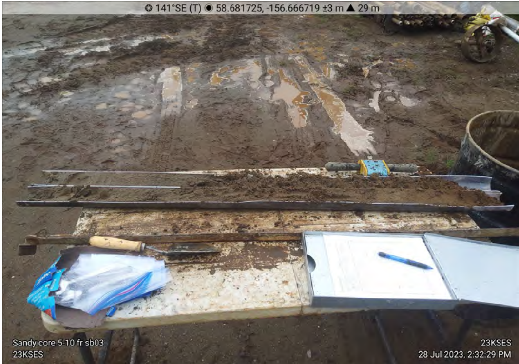
Photo 13. SB-03 5-10 ft bgs, sandy. Date: 7/28/2023..
