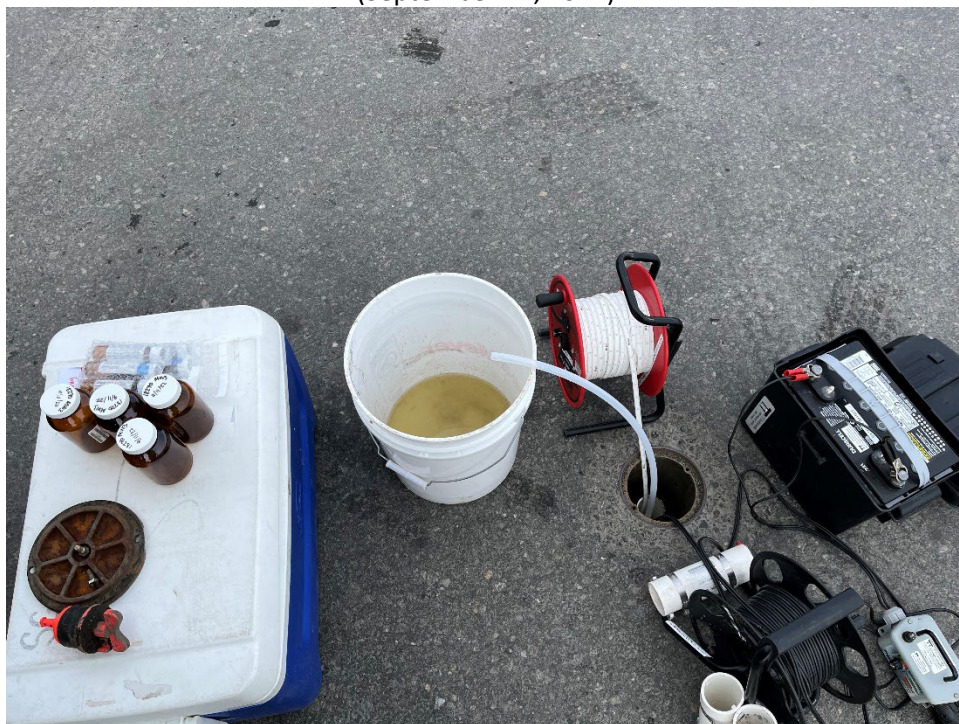
Photo 4: Monitoring Well Sampling. MW3 in source area, yellow water with odor. (September 11, 2022)
