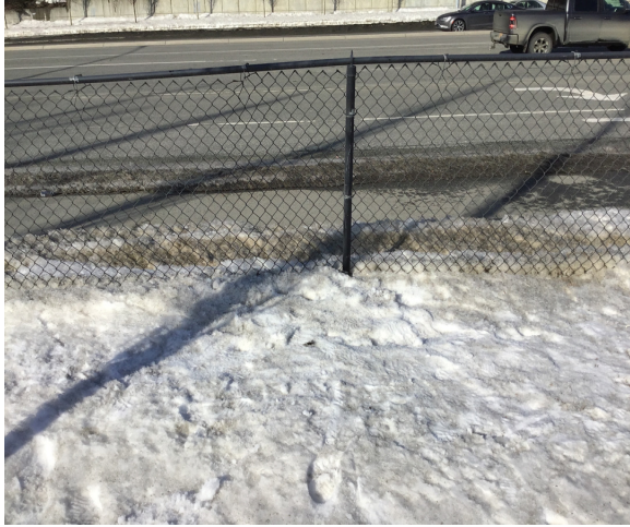
Approximate MW8RR location buried in roughly 2ft of ice, could not detect using magnetic locator because of close proximity to metal fencing
