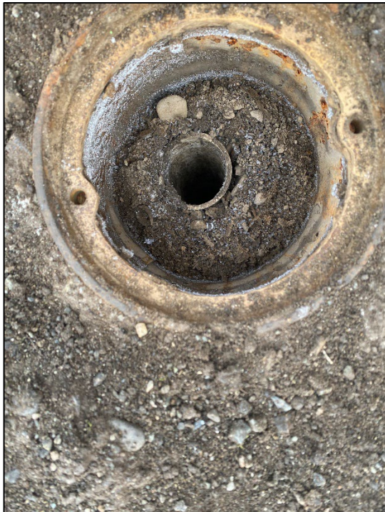
Photograph 6: View looking down. MW-124 opened with well cap off showing high soil level in the monument and dirt inside of the riser.
