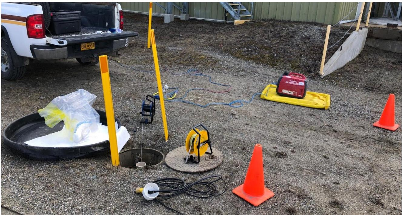
**Photo 2:** Recovering product at MW-5 after gauging depth to water and depth to product (June 7, 2022).
