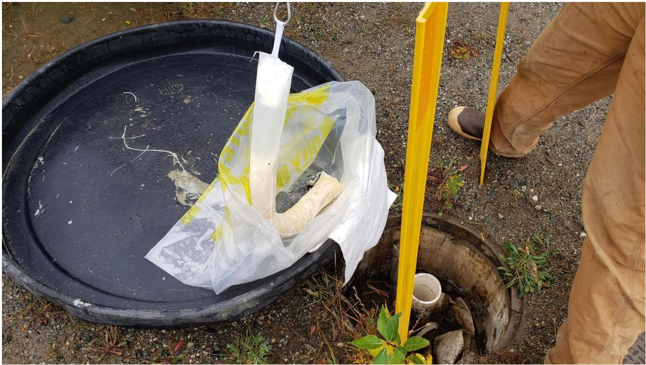
**Photo 3:** 4-inch sorbent recovered from MW-5. Product was recovered in the lower portion of the sorbent and an emulsion of water and product was recovered in the upper portion of the sorbent (September 20, 2022).
