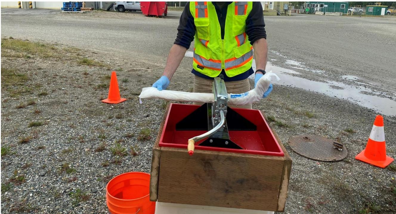
**Photo 2:** Running a 4" sorbent through the wringer. Product was collected in the red bin, and then emptied into a bucket prior to measurement in a graduated cylinder (August 11, 2020).
