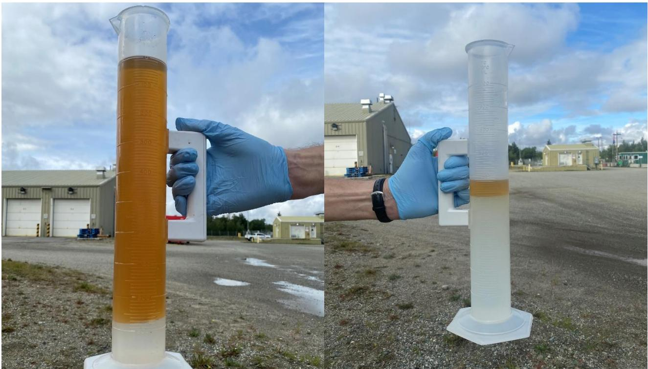
**Photo 4:** Two different photos showing variations in the ratio of product to water recovered by sorbents during different recovery events (left photo August 11, 2020; right photo August 25, 2020).
