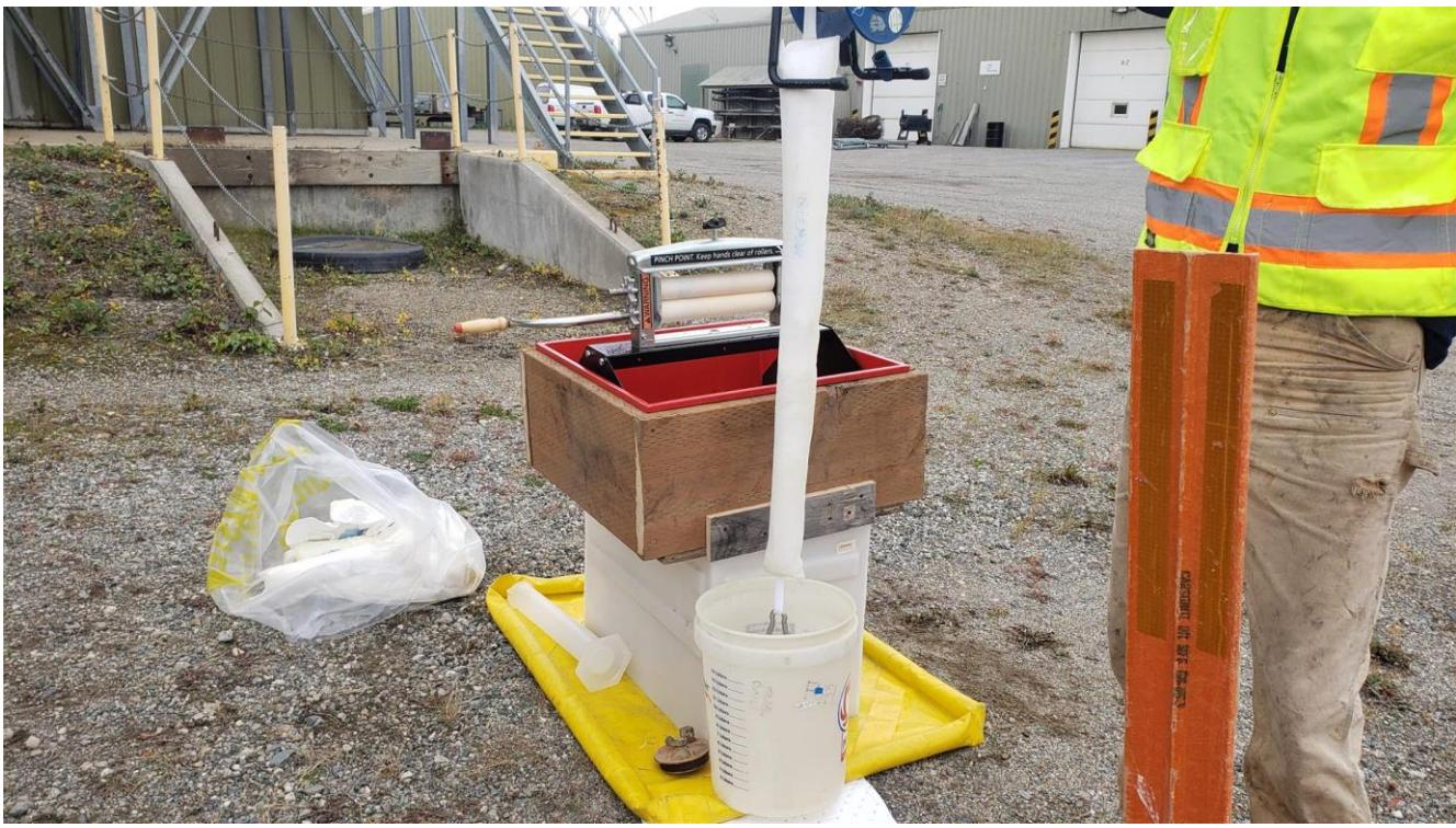
**Photo 1:** Draining excess product from a 4" sorbent before running the sorbent through a wringer (September 15, 2020).
