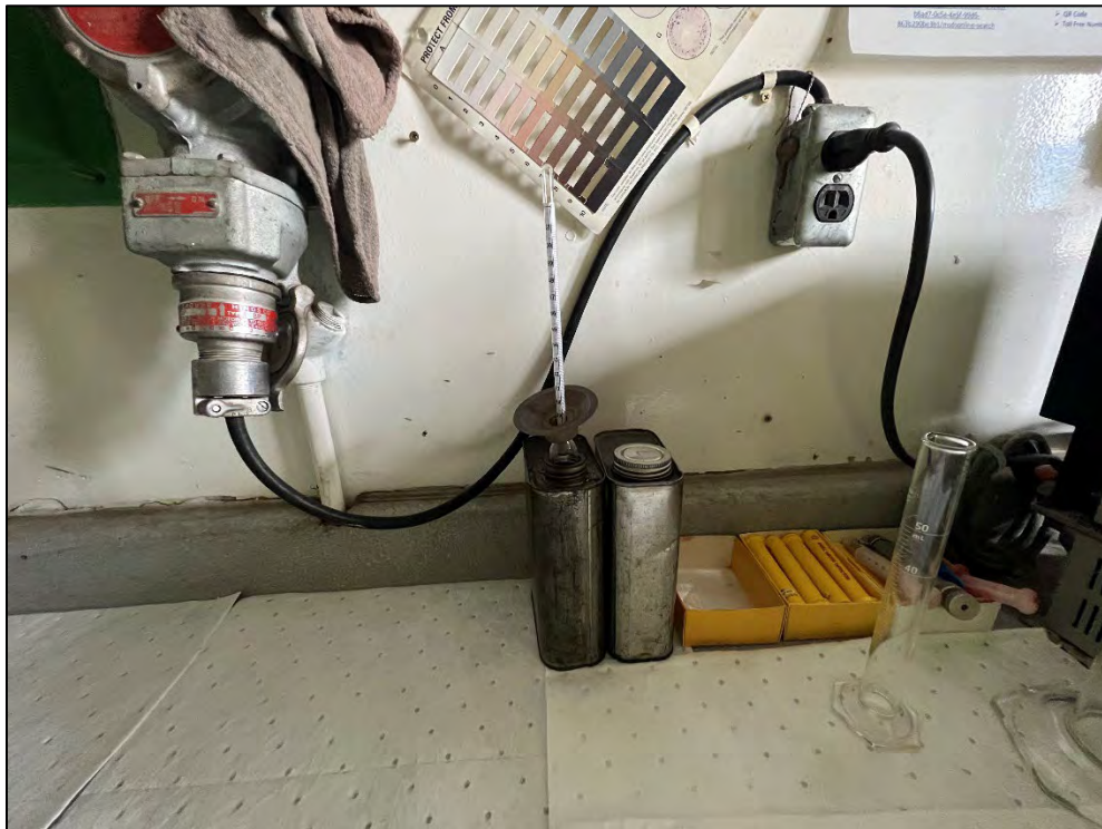
Photograph 11: View looking west. Close up on the metal sample containers at the flash point testing station in the back room.
