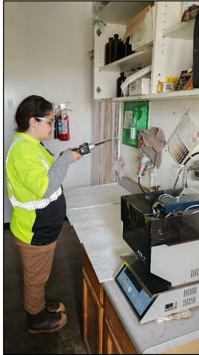
Photograph 44: View looking south. Collecting PID readings at the flash point testing station.
