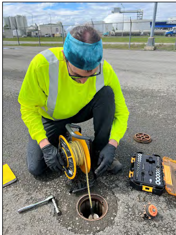
Photograph 4546: View looking west. Measuring water level at MW-4R.
