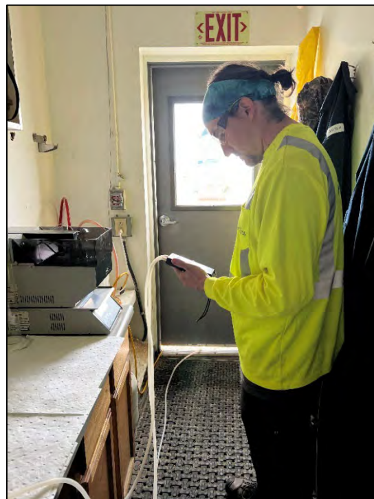
Photograph 41: View looking north. Collecting manometer readings at the north side of the building in the back room.
