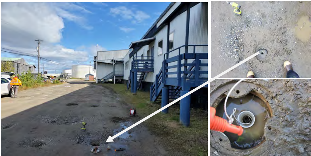
Photo 12: Monitoring Well MW6 located in a pothole along the school backroad. Water was originally above the well cap in the pothole. A sorbent sock, tied off to the well plug, was placed downhole. facing northeast. (August 15, 2022)
