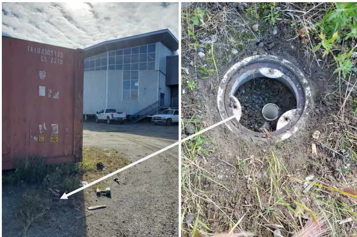
Photo 10: Monitoring Well MW5 located along a dirt road near a conex. facing south. (August 15, 2022)
