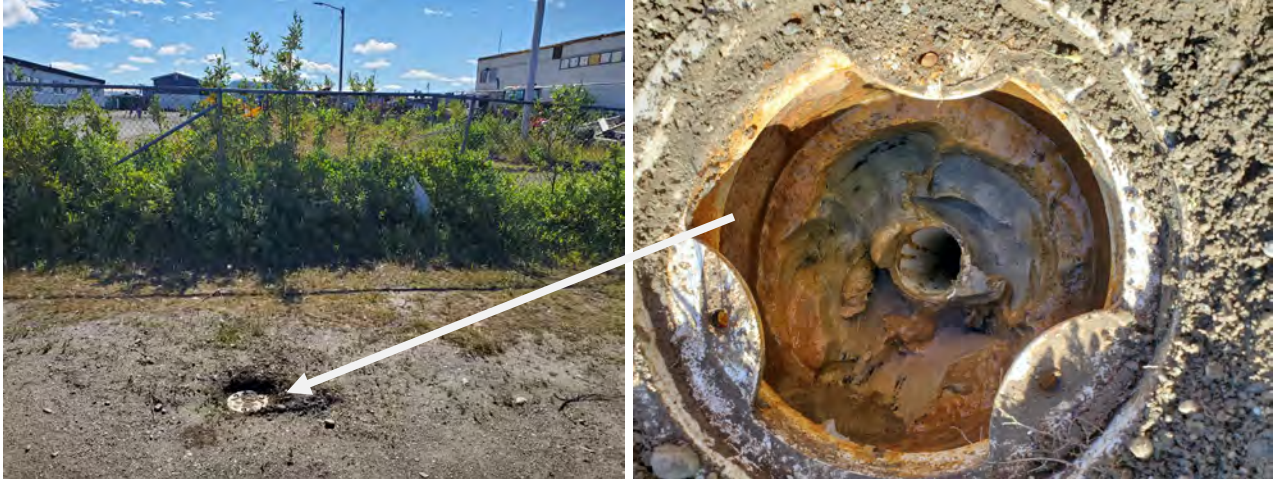
Photo 15: Monitoring Well MW9 located at the end of the road near the school. Bentonite had swelled above the well cap upon opening. (August 15, 2022)
