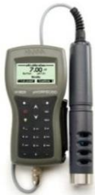
Photo 2: Hanna Multi-parameter Portable Water-Quality Meter (2013)
