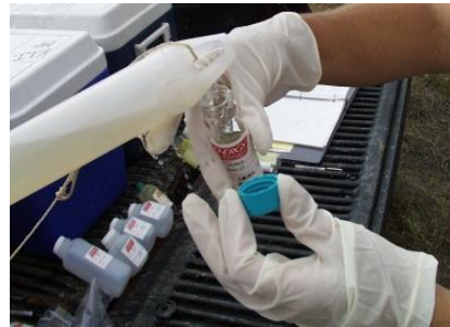
Photo 6: Filling VOA vials (TriHydro 2003)
