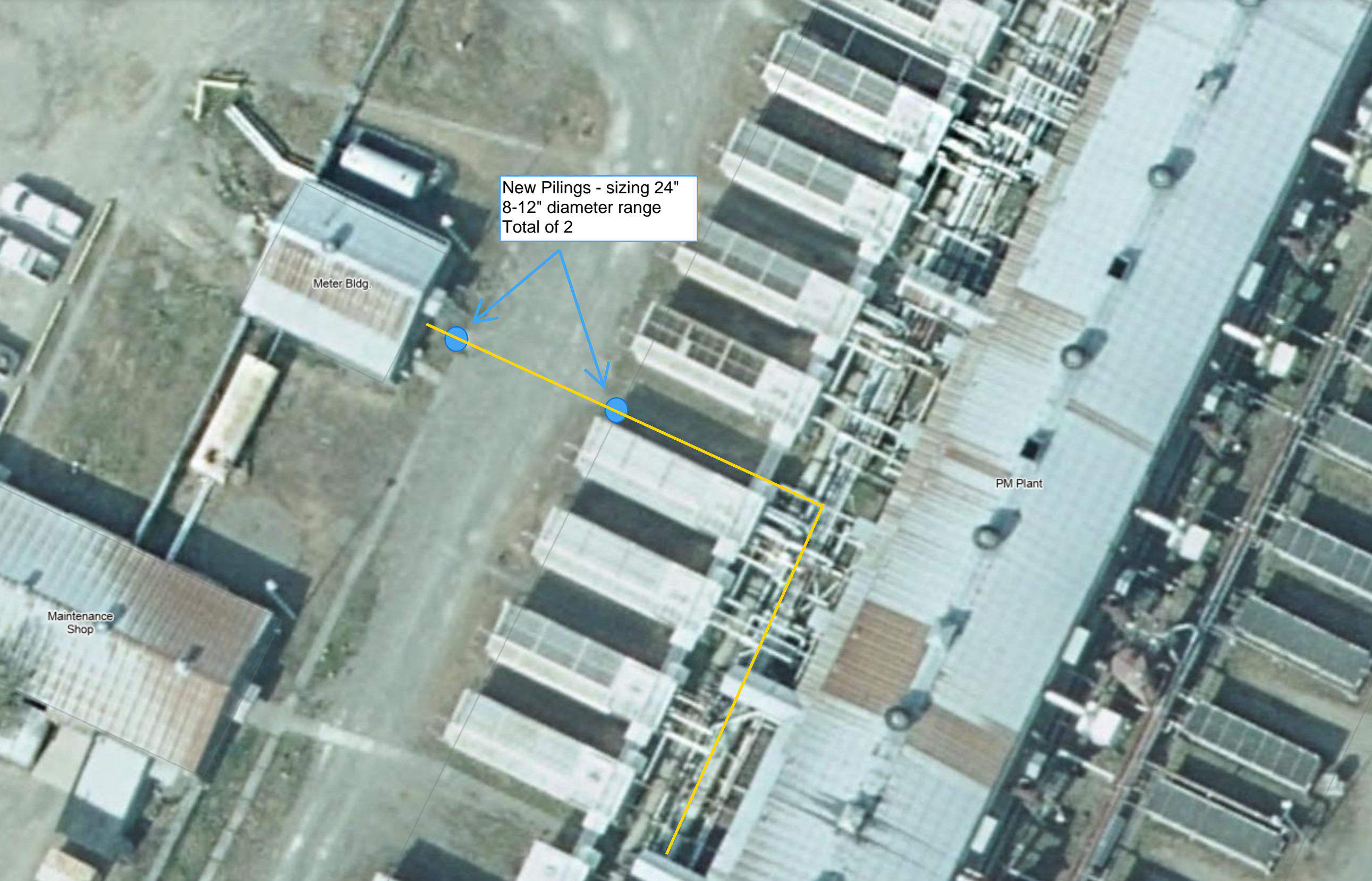
Figure 1: Location of New Piling for Above Ground Pipeline Supports, Swanson River Facility.
