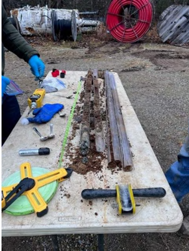
Photo 3, October 12, 2023 – Logging a soil core at Abandoned Diesel Tank Farm, looking southeast.
