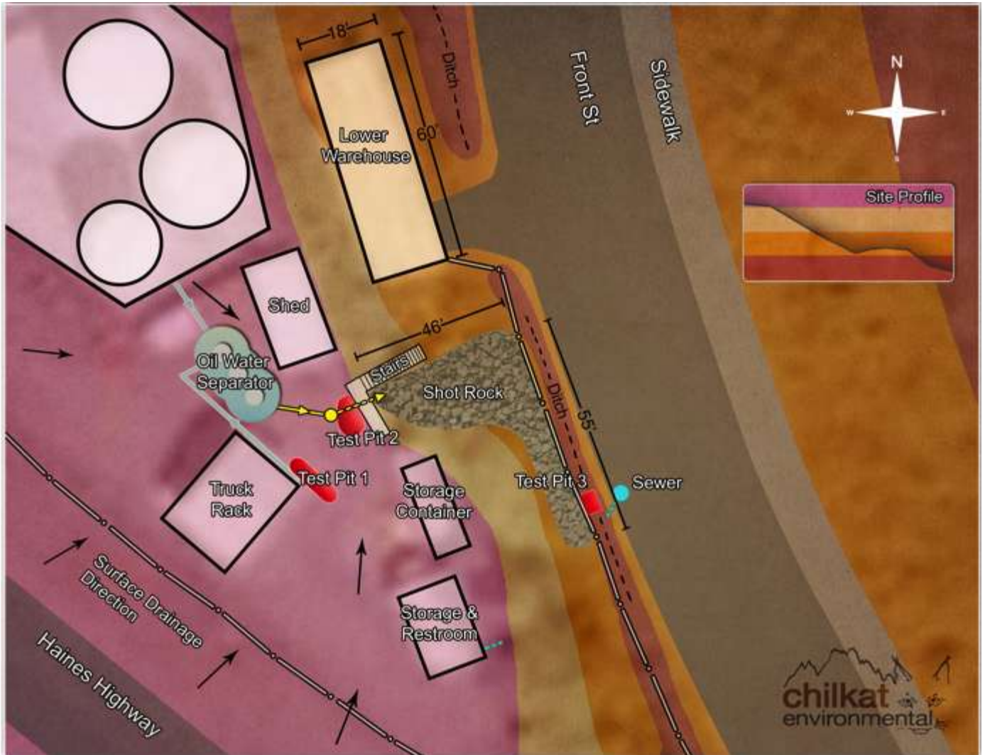
Figure 3: Site drawing featuring location of test pits. Site profile demonstrates approximated slope and surface drainage.
