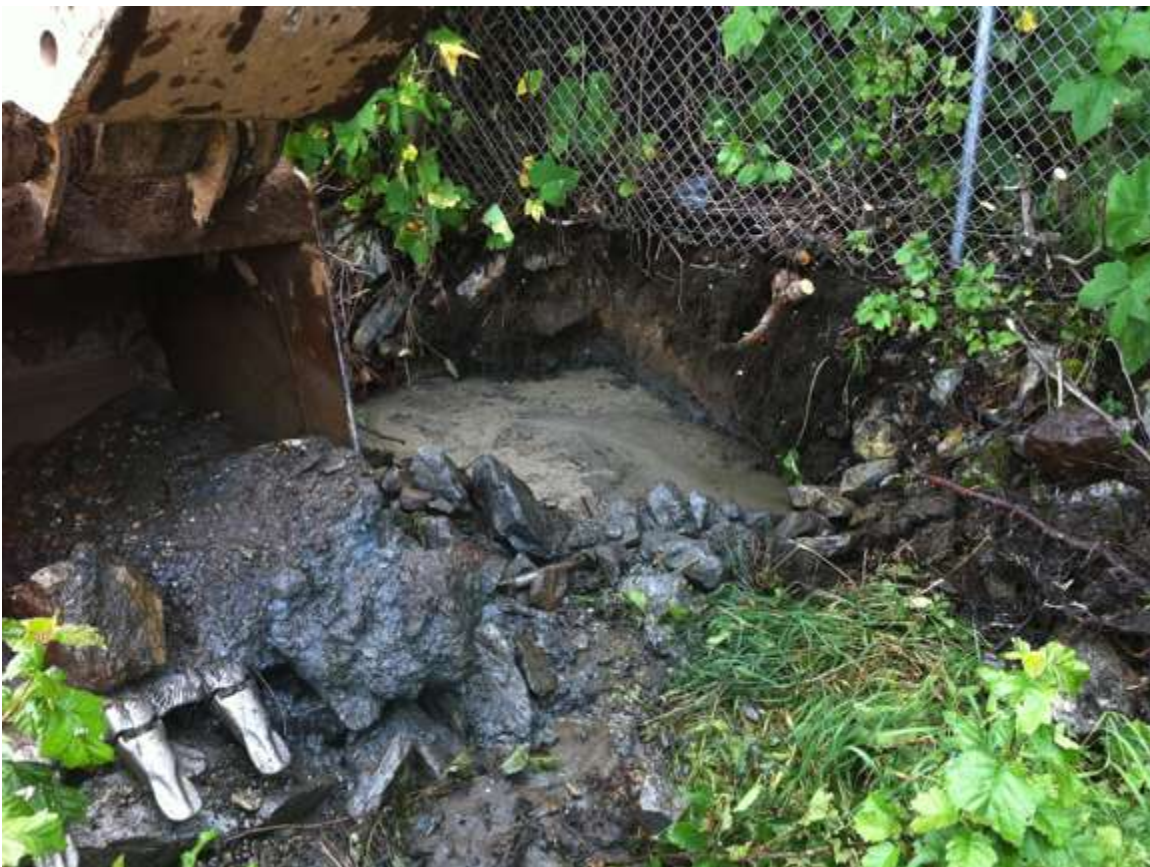
Photo 20: Test Pit #3 was only advanced 2 feet and encountered contaminated soil and shallow surface water featuring visible free product released by our disturbance.
