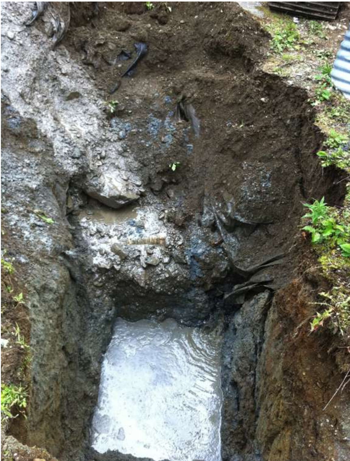
Photo 16: Test Pit #2 was advanced to 10 feet and no clay was encountered. The upper 2 feet featured clean soil while the rest of the soil column featured significant contamination. No groundwater was encountered. Excavation water sampled for Test Pit #2 originated from OWS and flowed into pit from outfall pipe.
