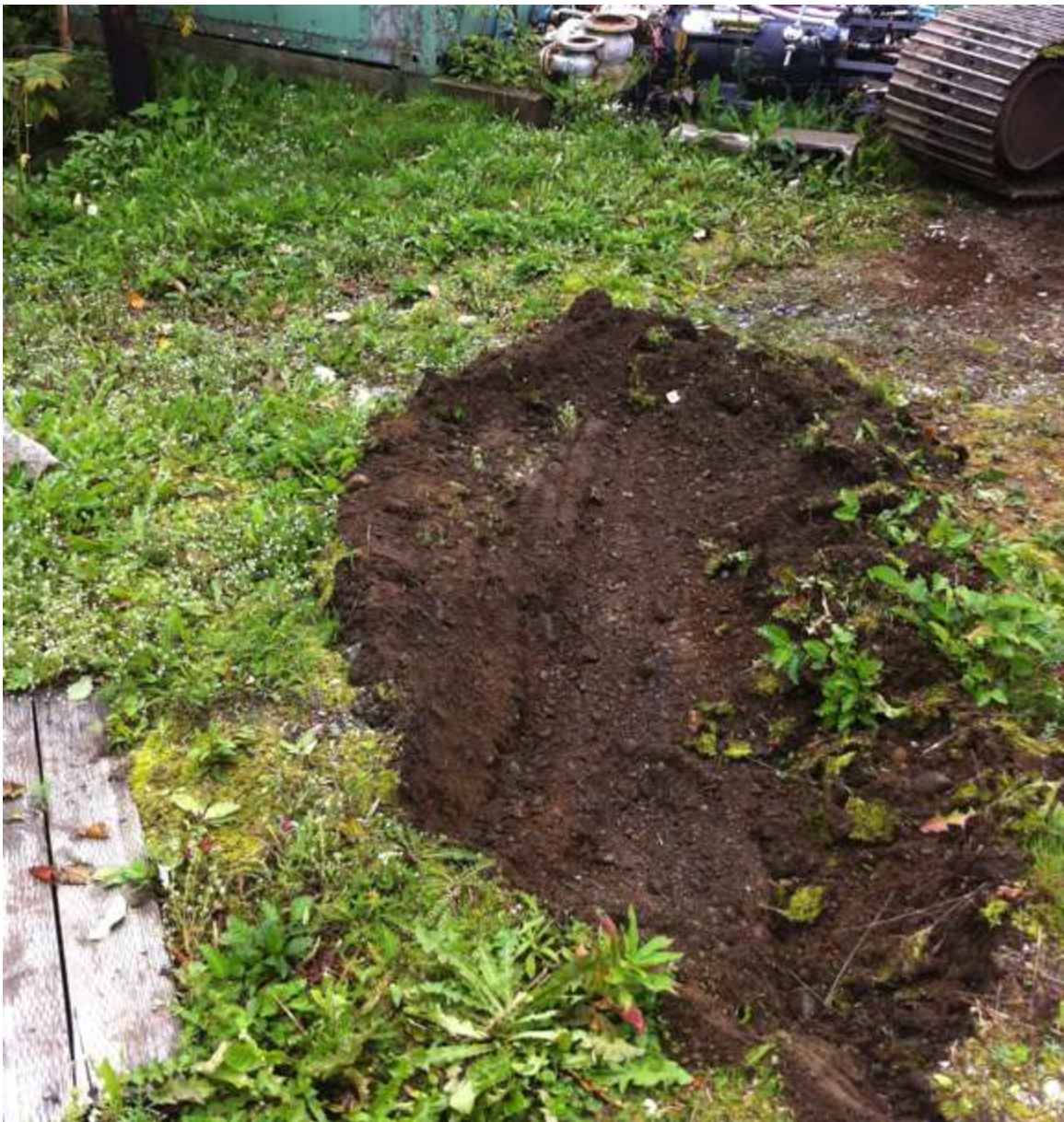
Photo 13: Test Pit #2 was forwarded directly between the oil water separator outfall and the stairway that accesses the Front Street.
