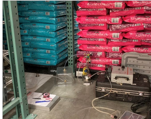
Photo 4-3: Collecting soil-gas sample SSV-1 near the south end of the Costco warehouse.
