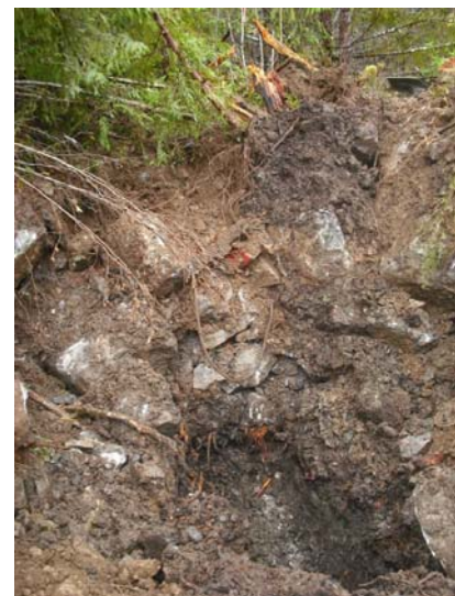
Photograph 6 ~ Rip Rap Encountered in Test Pit 2.
