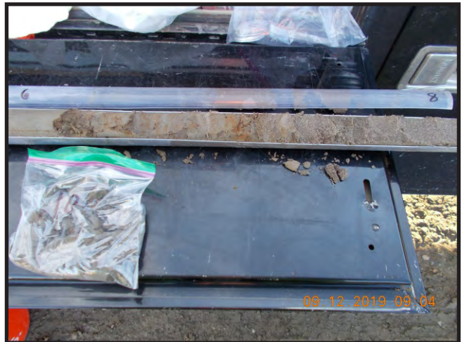
PHOTOGRAPH 4: CLOSE UP VIEW OF GEOPROBE SAMPLE CORE COLLECTED FROM BH2 FROM 6-8' BGS.
