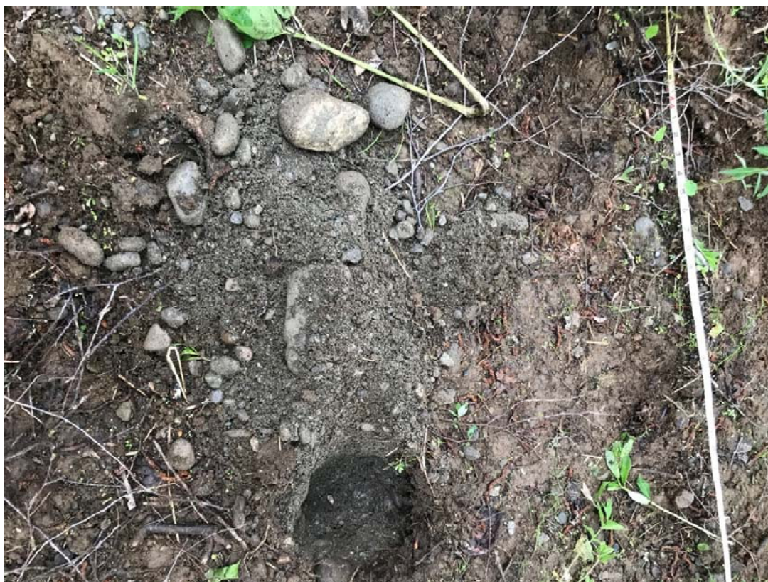
Grid 1 Soil Test Hole with Granular Material Visible
