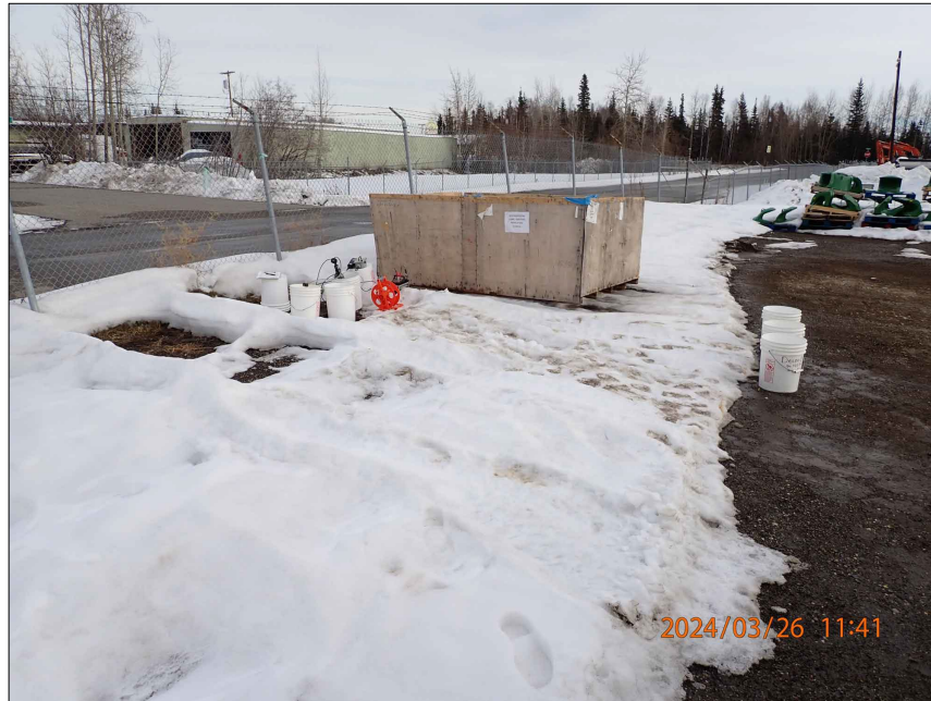
Photo 3: March 26, 2024. Looking northeast at MW-4 showing 20 th Avenue (background) as the well is purged using a low flow submersible pump. Water quality parameters were measured with a YSI Pro DSS instrument prior to groundwater sample collection.
