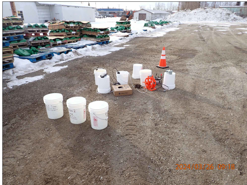
Photo 4: March 26, 2024. Looking southeast at MW-5 showing the CMI yard as the well is purged using a low flow submersible pump while water quality parameters are measured with a YSI Pro DSS instrument prior to groundwater sample collection. The 4-Bay Building is shown (upper left, background).
