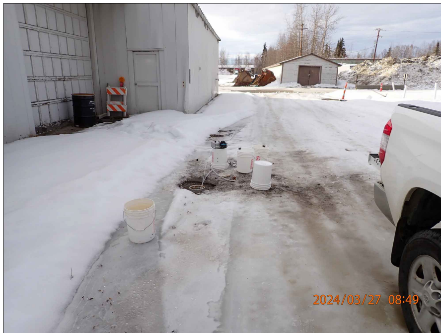
Photo 2: March 27, 2024. Looking south at MW-3 (center) showing the 4-Bay Building (left) as the well is purged using a low flow peristaltic pump instead of a submersible pump due to historic elevated contaminant concentrations. Three to five well volumes of water were removed prior to groundwater sample collection.
