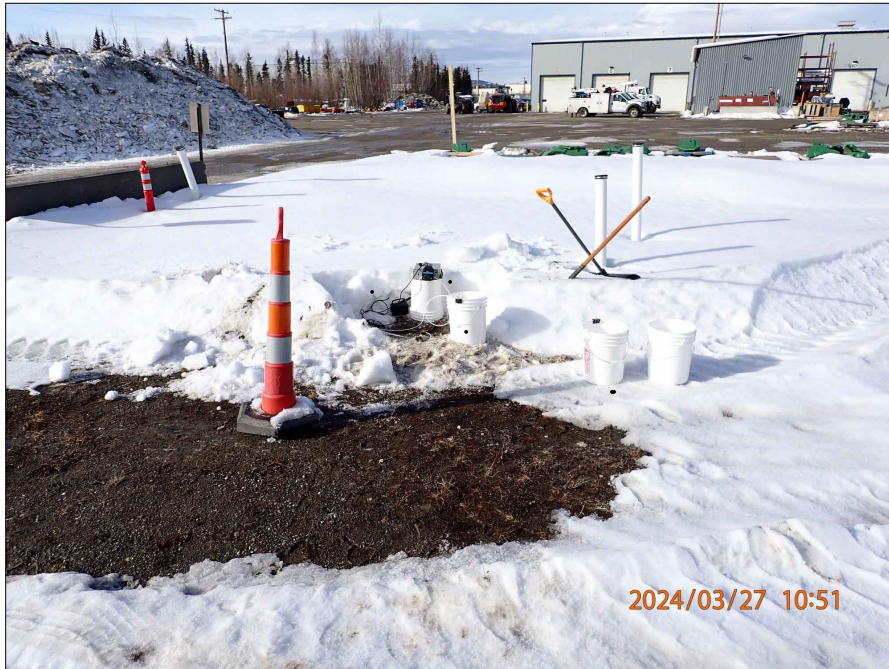
Photo 1: March 27, 2024. Looking west at MW-2 (center) showing the CMI facility (background) as the well is purged using a low flow peristaltic pump instead of a submersible pump due to historic elevated contaminant concentrations. Three to five well volumes of water were removed prior to groundwater sample collection.
