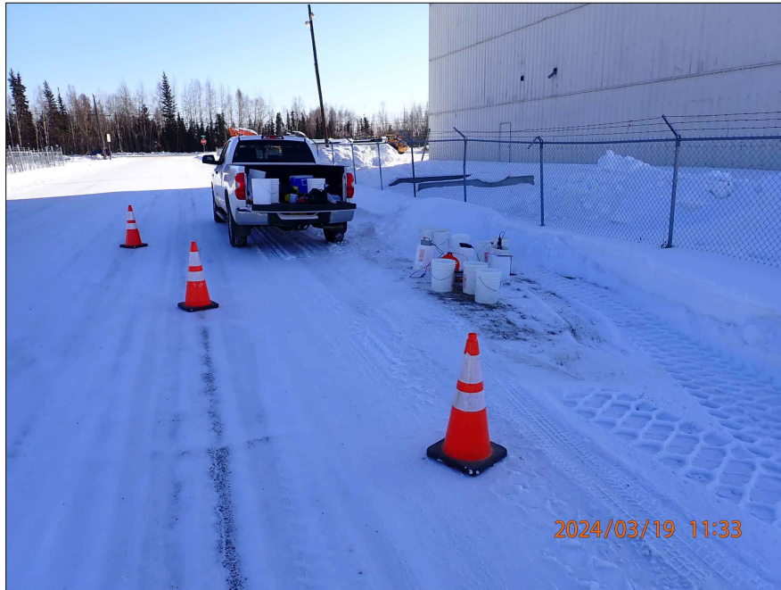
Photo 5: March 19, 2024. Looking east at MW-403A and MW-403B in 20 th Avenue ROW. The wells were purged using a low flow submersible pump while water quality parameters were measured with a YSI Pro DSS instrument prior to groundwater sample collection. The 2-Bay Building is shown on the right.
