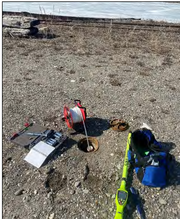
Photograph 2: 4/28/22. Measuring depth to water at MW-7R. View to north.
