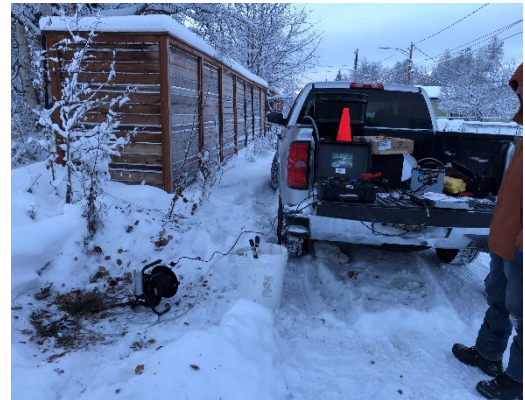
Photo 4-1: Purging monitoring well MW-9, in the Charles-Slater subdivision across Noyes Slough from the Bentley Mall.
