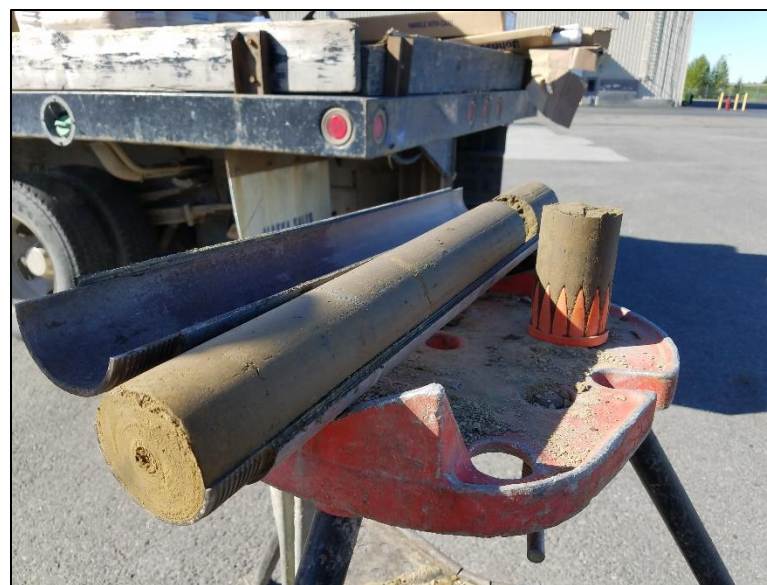
Example core of sandy silt with clay from RSE-1.
