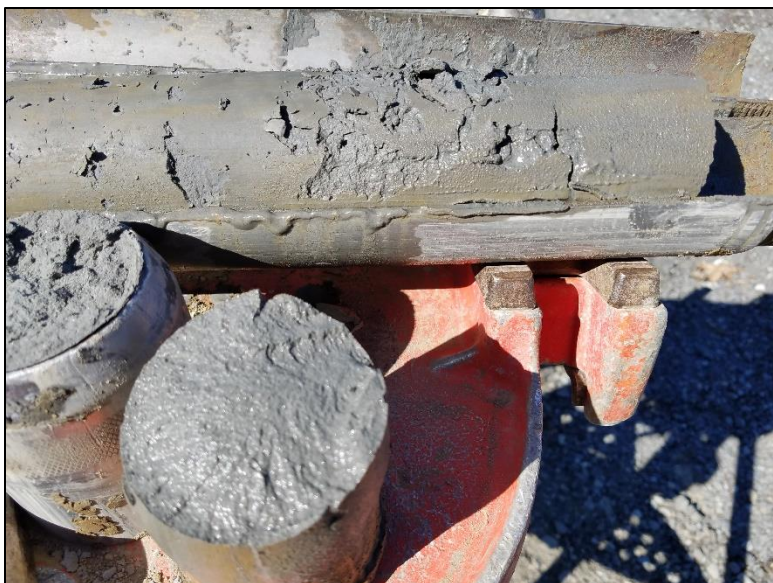
Example of drive interval containing dense sandy silt and clay.
