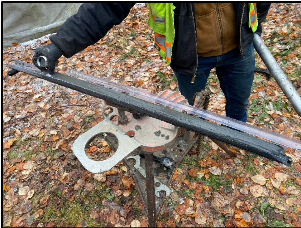
Photo 4: Soil boring showing saturated, very fine sand with strong petroleum
