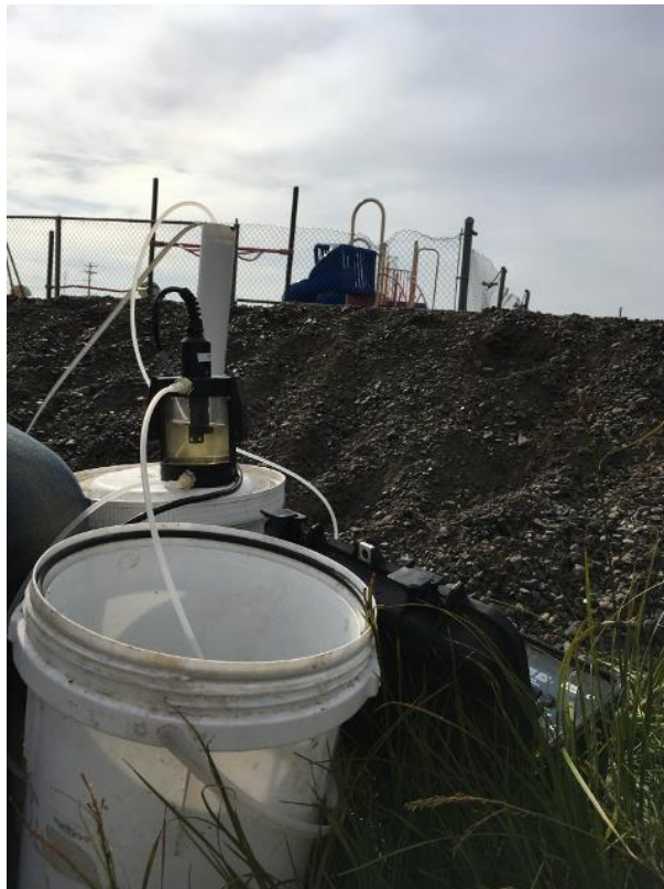
Photo 2: Groundwater Sampling MW-01
