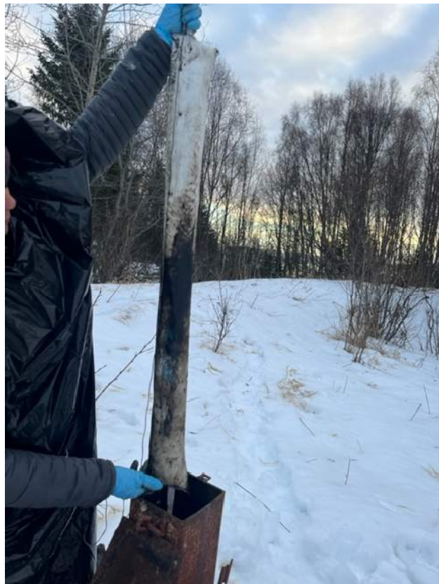
PHOTOGRAPH 8: Granite Point Production Facility MW7, absorbent sock. 16 November 2022.
