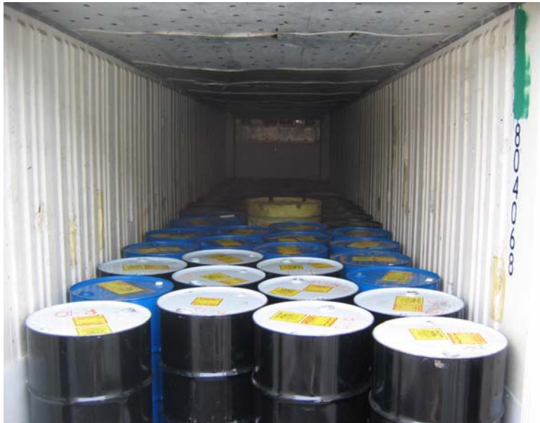
Photo 21: Inside of 40 foot container used for shipping dielectric oil and rinsate
