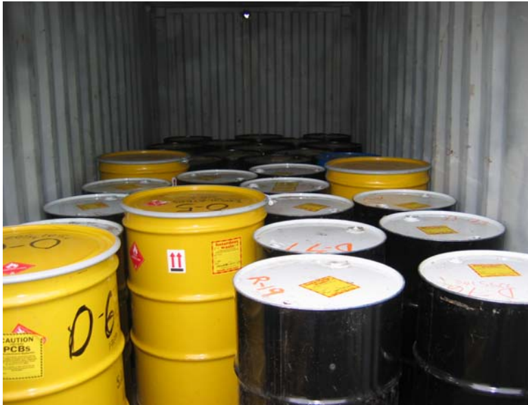
Photo 22: Inside of 20 foot container used to ship PCB waste and over 50ppm dielectric oil. A second layer of drums was added along with wood framing to hold drums in place.
