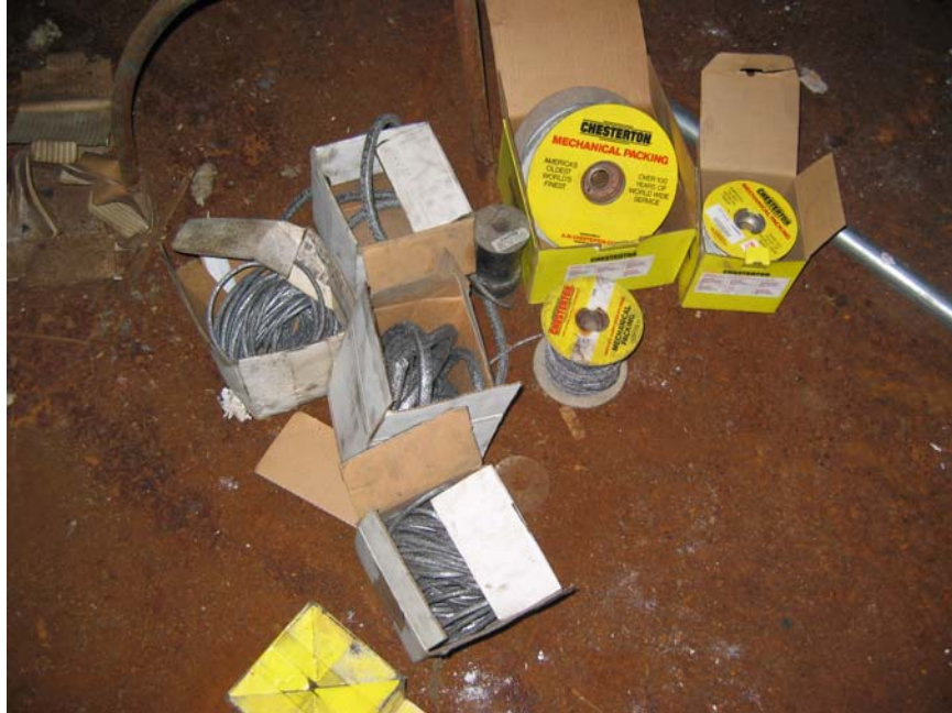
Photo 11; Mechanical Packing Material Labeled Asbestos on Second Floor
