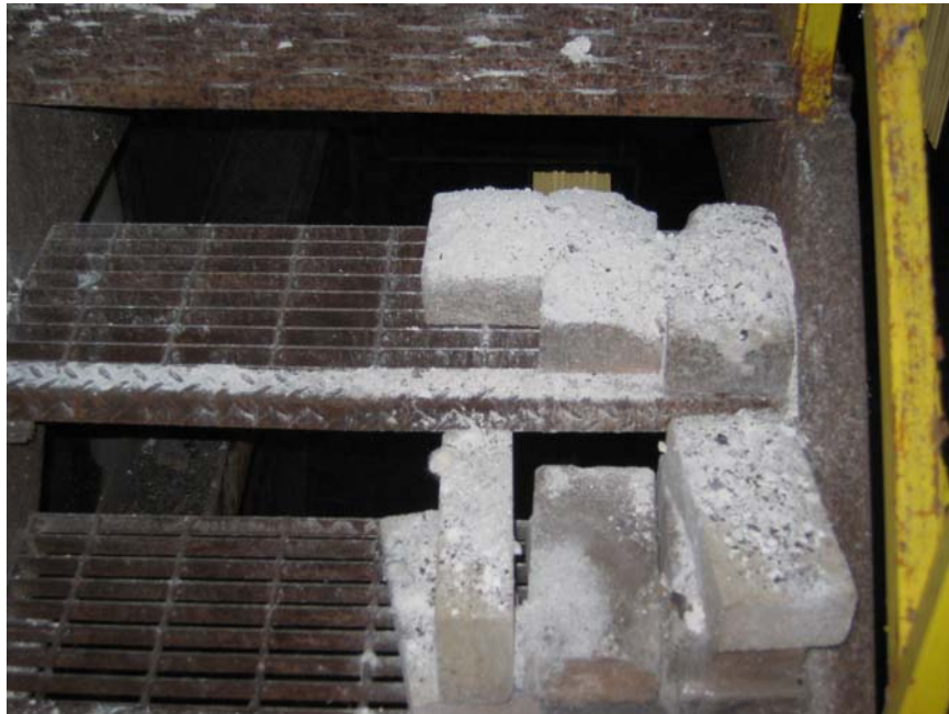
Photo 10: S-13 Diablo Bricks; Result Non-ACM
