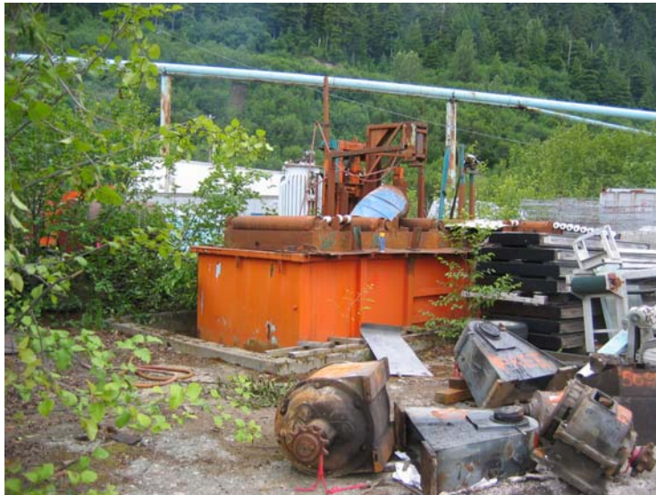
Photo #18: Dip Tank includes orange metal structure and concrete containment. Drained gear boxes are in the foreground destined for recycling
