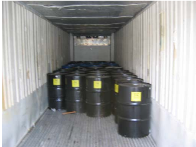
Photo 1: Trailer #1 includes Dielectric Fluid <50 ppm 38 drums and 1 overpack with gasoline contaminated at 5.87 ppm
